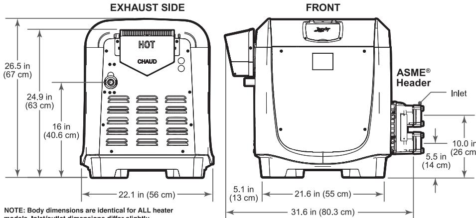
NOTE: Body dimensions are identical for ALL heater models. Inlet/outlet dimensions differ slightly.
